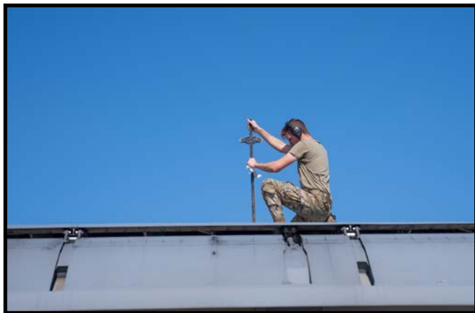
Staff Sgt. Tyler Bell dips the fuel tank to verify fuel level on a Nevada Air National Guard C-130 at Modular Airborne Fire Fighting System (MAFFS) Spring Training May 6, 2024 at Channel Islands Air National Guard Station in Port Hueneme, Calif.
